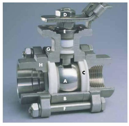
**Ball (A)** Flow-Tek balls are precision machined and mirror finished for bubble-tight shut off with less operating torque. Ball edges have machined curvatures to reduce seat wear and provide a high cycle life.
