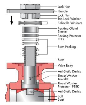
**Stem Packing** An adjustable V-ring design creates a multiple seal between the stem and body. Each stem assembly is composed of three or four (dependent on valve size) rings providing a very high cycle life by resisting creep and cold flow. The Thrust Washer and the Thrust Washer Protector combine to provide a primary seal, reduce torque and prevent galling. This arrangement is a Flow-Tek exclusive.
