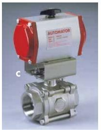
**Secure Mount (C)** The integrally cast top flange ensures positive actuator mounting. Secure Mount eliminates unwanted actuator movement during high cycle or continuous duty applications. Actuation equipment can be easily and safely removed while the valve is under full line pressure. Designed to ISO 5211 bolting pattern standards.
