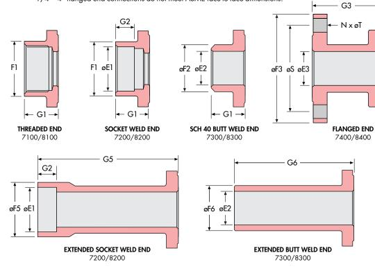
Flow-Tek's 3 piece valve is offered with a center body and a large selection of end connections. This versatile design offers easy customizing to meet most special application requirements.
