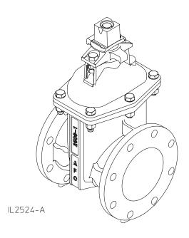
The **Series 2500 Ductile Iron** Resilient Wedge Gate Valve has a rated working pressure of 250 psig and is designed for use in drinking water, sewage, fire protection systems, and irrigation and backflow control systems.
