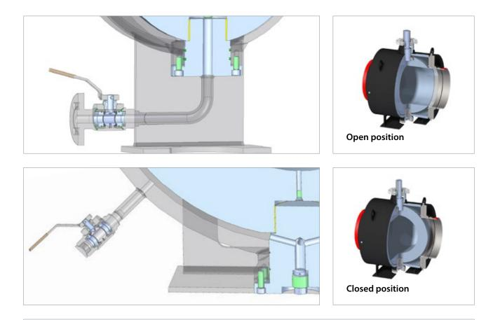
BROEN Ballomax<sup>®</sup> can be delivered with DBB outlet valve placed different places on the valve body. BROEN Ballomax<sup>®</sup> Trunnion is delivered with DBB outlet at the bottom as standard. The drain allows the pressure in the cavity to be released manually, as well as the tightness of the valve to be checked, without the need to shut down the pipeline.
